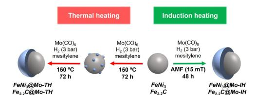
Scheme 1 Schematic representation of thermal and magnetically induced molybdenum coating on magnetic nanoparticles.
