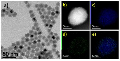
Fig. 2 Fe<sub>2.2</sub>C@Mo-TH NPs, (a) BF TEM image, (b) STEM-HAADF image and STEM-EDX mapping showing (c) Fe (blue), (d) Mo (green), and (e) overlap of Fe and Mo maps
