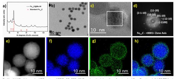
Fig. 3 Fe<sub>2.2</sub>C@Mo-IH NPs, (a) powder XRD pattern (ICDD: 00-036-1249, red vertical drop lines for standard Fe<sub>2.2</sub>C pattern), (b) BF TEM micrograph, (c) HRTEM image, (d) FFT pattern derived from the white square marked zone of image c along (0001) zone axis, (e) STEM-HAADF image, (f)-(h) STEM-EDX elemental maps showing Fe in blue and Mo in green, and overlap of Fe and Mo maps.
