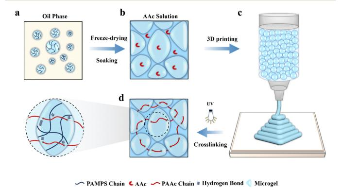
Fig. 1 PAMPS microgels for 3D printing. (a) PAMPS microgels are prepared by inverse emulsion polymerization, (b) followed by soaking in AAc solution to produce a highly swollen and jammed microgel ink (c) for extrusion-based 3D printing various microstructures; (d) post-printing curing by UV light generates a PAAc network interpenetrating throughout the PAMPS microgels, yielding microgel-reinforced double network (MRDN) hydrogel constructs with different microstructures.
