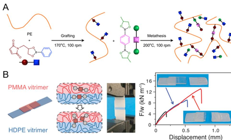
**Fig. 15** (A) Conversion of commercial HDPE to vitrimers *via* metathesis with dioxaborolane. (B) Adhesion between the two vitrimers is also enhanced due to the presence of dynamic dioxaborolane bonds. Reproduced in part with permission from ref. 41. Copyright 2017 *Science*.
