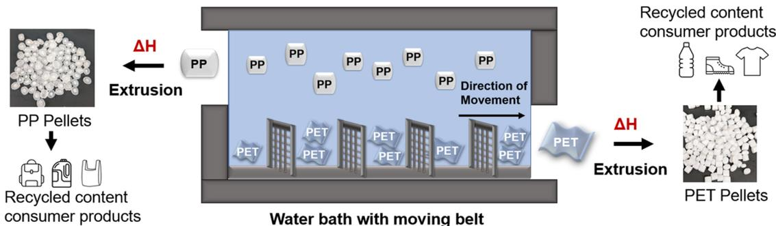
Fig. 4 Difference in density can be used to sort plastic types (PET vs. PP) in a water bath. Once the plastics have been sorted by type, they can be processed separately and then heated and extruded into pellets to be made into recycled content containing consumer products.
