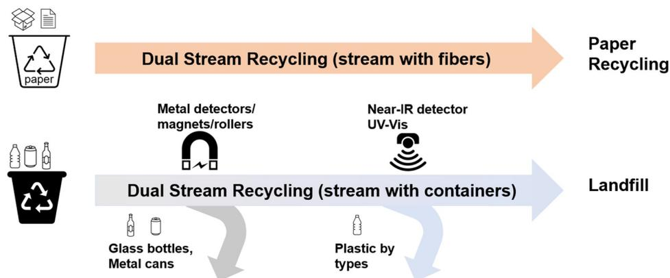
Fig. 2 Single stream vs. dual stream recycling feedstock, where the single stream contains all recyclable materials while the dual stream separates materials such as paper and cardboard from glass, metals, and plastics.
