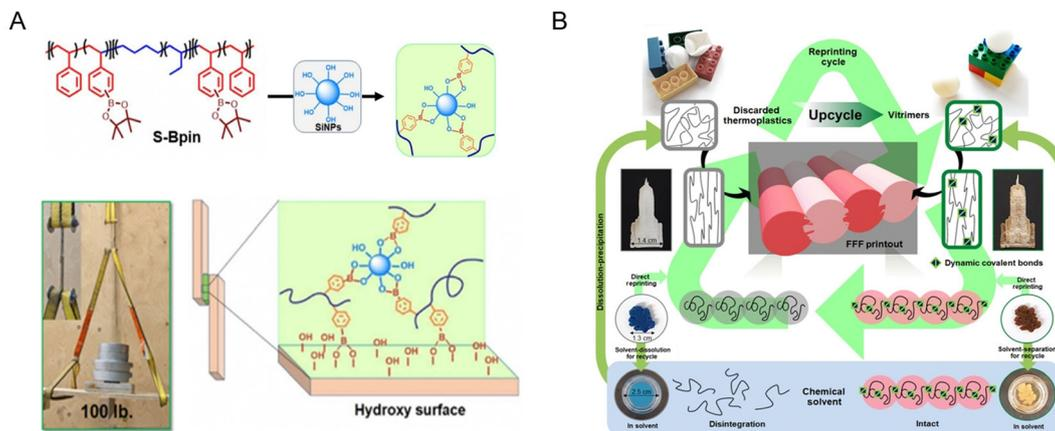
Fig. 16 (A) Tough adhesive from upcycled commodity polymer SEBS. (B) Closed-loop additive manufacturing *via* upcycled ABS vitrimers. The photographs show structures printed from the untreated ABS (Neat-ABS) (left) and the ABS-vitrimer (right) of a building (top) and an oak leaf before (middle) and after (bottom) immersion in tetrahydrofuran (THF) for 48 hours. Reproduced with permission from ref. 42 and 43. Copyright 2021 *Sci. Adv.* and 2022 *Sci. Adv.*
