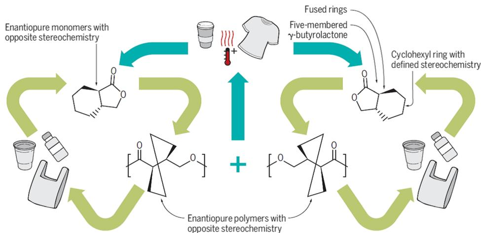
Fig. 10 Polymers synthesized from  $\gamma$ -butyrolactone exist as two enantiomers and when blended, this allows for materials with improved thermal stability which can be recycled repeatedly without losing mechanical properties. Reproduced with permission from ref. 28. Copyright 2018 Science.
