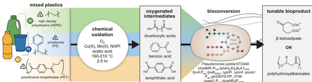
Fig. 9 Upcycling of mixed plastic waste through tandem chemical oxidation and bioconversion. Metal-promoted autoxidation simultaneously deconstructs multiple polymers, generating a mixture of oxygenated intermediates that are advantageous substrates for bioconversion. An engineered *P. putida* strain funnels the heterogeneous mixture of oxygenates into a single target product. Reproduced with permission from ref. 25. Copyright 2022 Science.
