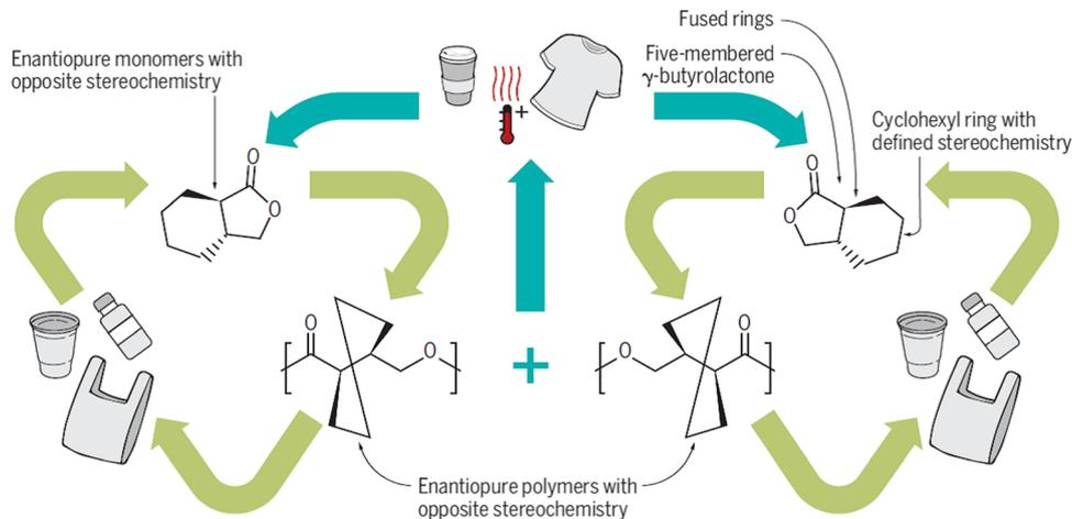
Fig. 10 Polymers synthesized from  $\gamma$ -butyrolactone exist as two enantiomers and when blended, this allows for materials with improved thermal stability which can be recycled repeatedly without losing mechanical properties. Reproduced with permission from ref. 28. Copyright 2018 Science.
