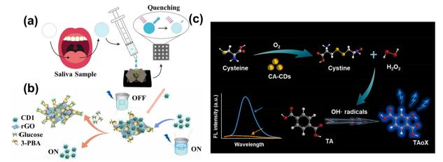
Fig. 8 (a) The schematic diagram of CDs sensing glucose and lactate in saliva samples.<sup>114</sup> Reproduced from ref. 69 with permission from Elsevier, copyright 2021. (b) The illustration of the preparation of rGO-PBA and use in detecting glucose. 116 Reproduced from ref. 71 with permission from Elsevier, copyright 2022. (c) The schematic image of CA-CDs detecting cysteine through oxidation. 117 Reproduced from ref. 72 with permission from Elsevier, copyright 2022
