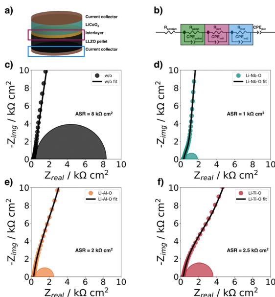
Fig. 5 (a) Schematic of half-cells structure for electrochemical impedance spectroscopy at room-temperature, (b) equivalent circuit model used to fit the impedance spectra by Zhang *et al.*,<sup>43</sup> EIS spectra of (c) Au|LCO|LLZO|Au (w/o), (d) Au|LCO|Li–Nb–O|LLZO|Au (Li–Nb–O), (e) Au|LCO|Li–Al–O|LLZO|Au (Li–Al–O), and (f) Au|LCO|Li–Ti–O|LLZO|Au (Li–Ti–O). The measured data are shown together with the fits from the equivalent circuit.
