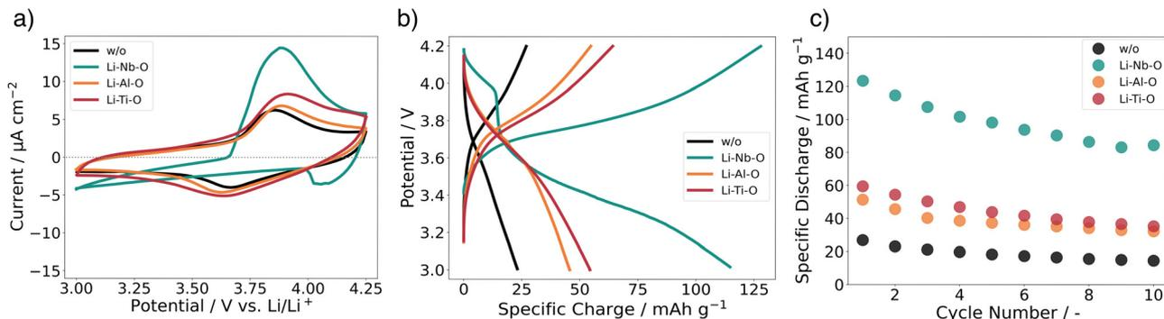
Fig. 6 (a) Cyclic voltammograms measured with a sampling rate of  $0.1 \text{ mV s}^{-1}$  between 3 and 4.25 V vs.  $\text{Li/Li}^+$ , (b) charge–discharge curves with  $1.75 \mu\text{A cm}^{-2}$  between 3 V and 4.2 V at  $80^\circ\text{C}$ , and (c) specific discharge capacities for full cells with and without interface modification.
