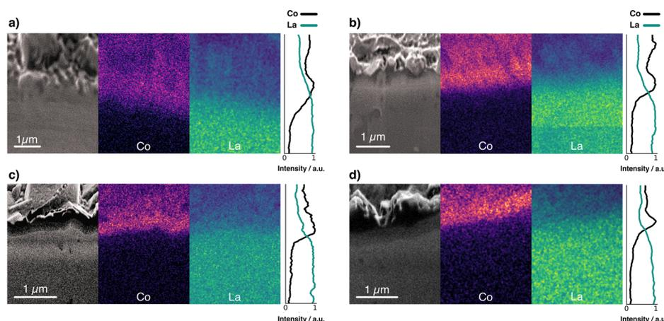
Fig. 4 FIB-SEM image and elemental mapping of Co K series and La L series of a stack (a) without interlayer, and with (b) Li–Nb–O, (c) Li–Al–O, and (d) Li–Ti–O interlayer.
