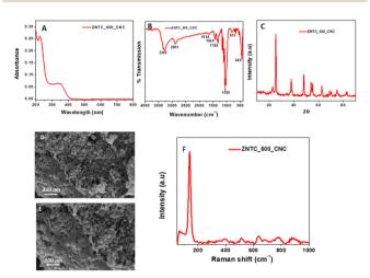
Fig. 2 Characterization of the cotton nanocellulose (CNC) and ZNTC\_600 composite. (A) UV-Vis spectrum. (B) FTIR spectrum. (C) XRD diffractogram. (D) and (E) Scanning electron microscope images. (F) Raman spectrum
