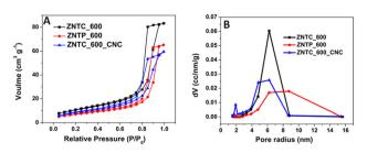
Fig. 9 (A) N<sub>2</sub> adsorption-desorption isotherms, and (B) pore radius distributions of ZNTC\_600, ZNTP\_600, and ZNTC\_600\_CNC
