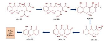
Fig. 8 The possible degradation pathway and intermediate products of TC-HC degradation
