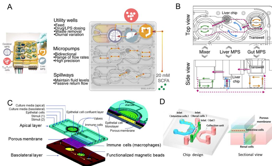
**Fig. 8** Microfluidic models of the gut-x axes. (A) Design, features, and parameters of the gut–liver–brain platform.<sup>56</sup> (B) Top and side view of the model of the human gut–liver axis, including adaptive immune cells.<sup>117</sup> (C) Schematic of the microfluidic chip forming the miniaturized gastrointestinal tract.<sup>118</sup> (D) Schematic of the multi-layered intestine–kidney chip.<sup>119</sup>
