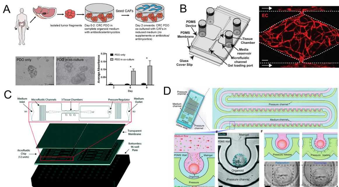
**Fig. 12** Organoids/organs-on-a-chip platforms for cancer research. (A) Schematic illustration of co-culture of CRC PDO and CAFs. Brightfield images and growth profile of PDO only and PDO in co-culture.<sup>164</sup> (B) Schematic of the vascularized micro-organ platform.<sup>165</sup> (C) The diagram of the vascularized micro-tumors microfluidic platform.<sup>166</sup> (D) The diagram of colon tumor organoids on the microfluidic platform with periodic movement.<sup>107</sup>
