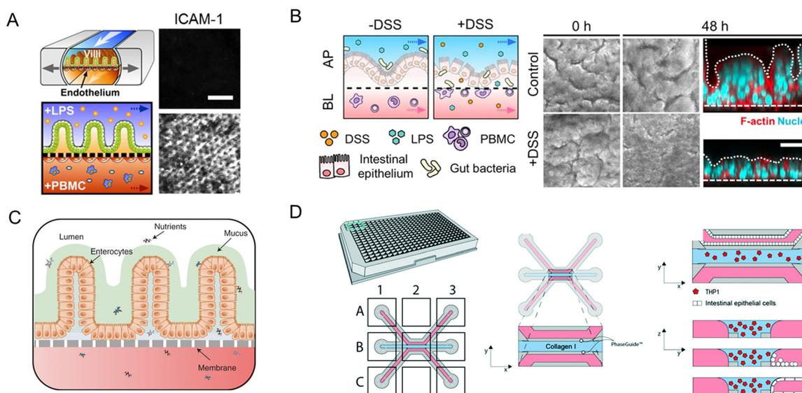
**Fig. 11** Organoids/organs-on-a-chip platforms to study intestinal autoimmune diseases. (A) Human intestinal inflammation and bacterial overgrowth.<sup>53</sup> (B) The diagram of DSS-mediated epithelial barrier dysfunction and morphology of the villus epithelium.<sup>89</sup> (C) The diagram of the EED chip model.<sup>13</sup> (D) Schematic representation of the intestinal mucosal barrier with cellular innate immunity.<sup>160</sup>
