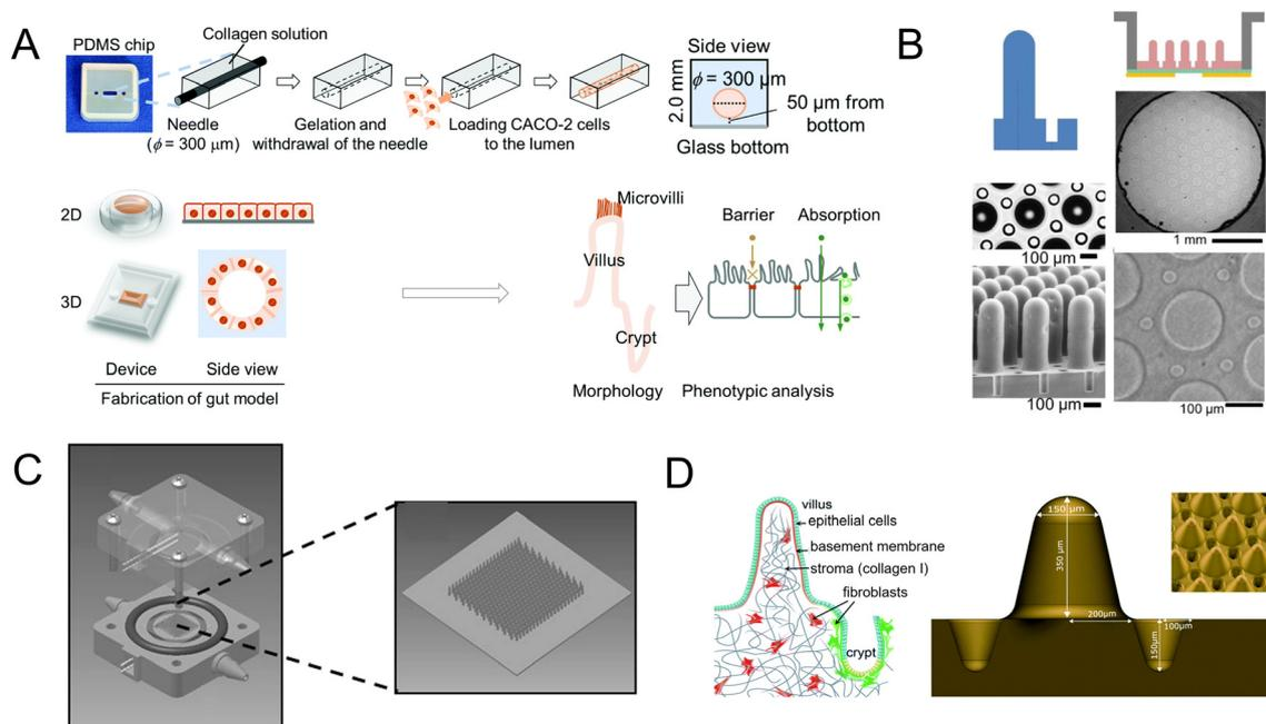
**Fig. 4** Mimicking intestinal surface topography on the chip. (A) Fabrication of the ductal scaffold of collagen gel.<sup>62</sup> (B) Micromolding a collagen scaffold employing a suitable extracellular matrix and stiffness.<sup>63</sup> (C) Scheme of the scaffold which is similar to the intestinal local villus surface topography.<sup>64</sup> (D) Fabrication of the biomimetic scaffold of 3D collagen scaffold guided stromal cells into the organoids-on-a-chip platform.<sup>65</sup>
