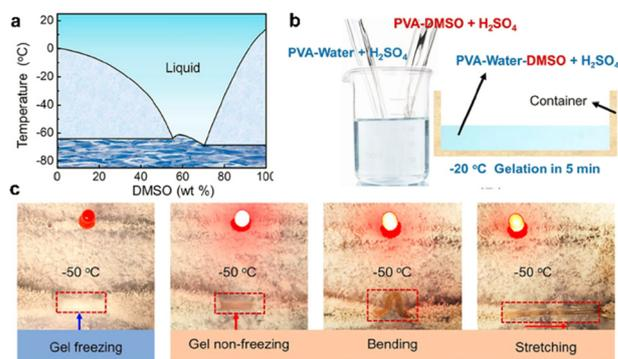
**Fig. 14** (a) Phase diagram of a mixed solution of water and DMSO. (b) The fabrication process of freeze-tolerant ionic skin based on the mixed solvent of water and DMSO. (c) This ionic skin can still light LED lights at  $-50\text{ }^{\circ}\text{C}$ . Reproduced with permission from ref. 82, copyright 2021, Wiley-VCH.
