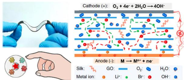
**Fig. 13** Humidity-sensitive chemoelectric flexible ionic sensors for noncontact perception. Reproduced with permission from ref. 66, copyright 2022, Nature Publishing Group.
