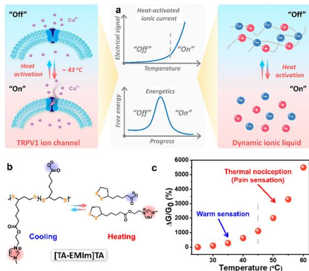
**Fig. 7** (a) Design concept of a TRPV1-like heat-activated dynamic ionic liquid; (b) the reversible conversion of the dynamic ionic liquid between the polymerized state and the monomeric state; (c) the electrical response of [TA-EMIm]TA at different temperatures. Reproduced with permission from ref. 11, copyright 2022, American Chemical Society.
