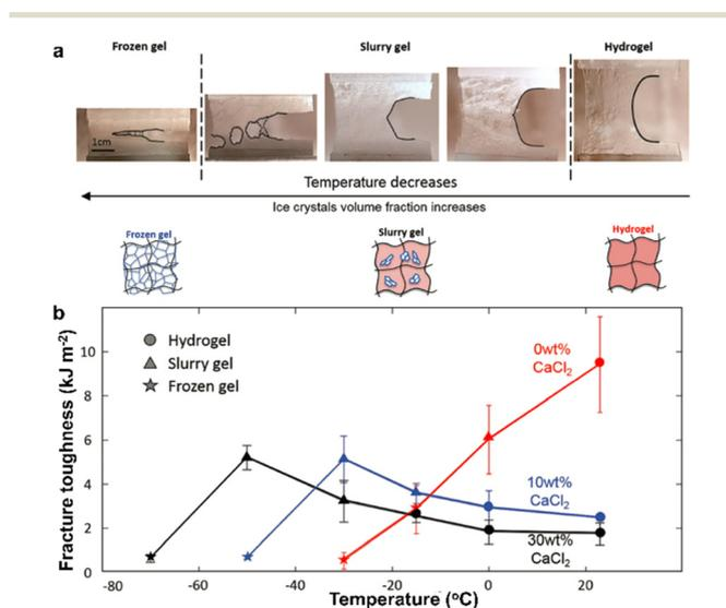
**Fig. 15** (a) Crack growth process of a hydrogel containing calcium chloride during the cooling process. The hydrogel consists of three stages: 1) regular hydrogel; 2) slurry gel; 3) frozen gel. (b) The fracture toughness of hydrogels with different calcium chloride contents at sub-zero temperatures. Reproduced with permission from ref. 83, copyright 2018, Wiley-VCH.
