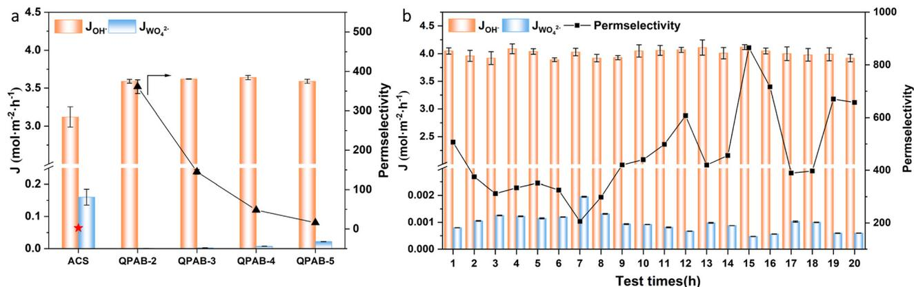
Fig. 7 (a) Anion fluxes and permselectivities of the Neosepta ACS and QPAB-*x* membranes in a NaOH/Na<sub>2</sub>WO<sub>4</sub> system at a current density of 10 mA cm<sup>-2</sup>; (b) operational stability of the QPAB-2 membrane for continuous ion selectivity.
