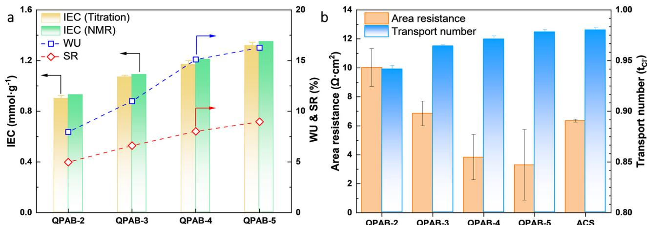
Fig. 3 Physical and electrochemical characteristics of QPAB-*x* and Neosepta ACS membranes. (a) IEC, WU and SR of QPAB-*x* membranes; (b) area resistance and transport number of QPAB-*x* and Neosepta ACS membranes.
