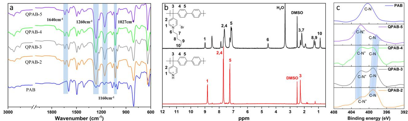
Fig. 1 Chemical structure analysis of PAB polymer and QPAB-*x* membranes. (a) ATR-FTIR spectra of PAB polymer and QPAB-*x* membranes; (b)  $^1\text{H}$  NMR spectra of PAB and the QPAB-2 membrane; (c) XPS spectra of PAB polymer and QPAB-*x* membranes.
