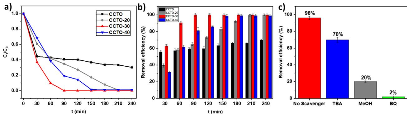
Fig. 7 (a) PCM degradation by electrocatalysis via PMS activation. (b) PCM removal efficiency. (c) Radical scavengers test. TBA: *tert*-butanol ( $\cdot\text{OH}$  scavenger); MeOH: methanol ( $\cdot\text{OH}$  and  $\cdot\text{SO}_4^-$  scavenger); BQ: *p*-benzoquinone ( $\cdot\text{O}_2^-$  scavenger).
