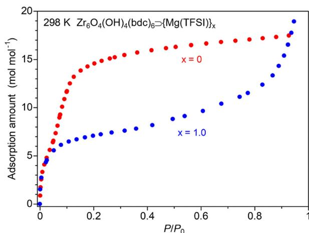
Fig. 4 Adsorption isotherms of blank UiO-66 ( $x = 0$ ) and UiO-66  $\Delta$   $\{Mg(TFSI)_2\}_{1.0}$  ( $x = 1.0$ ) under MeOH vapor.
