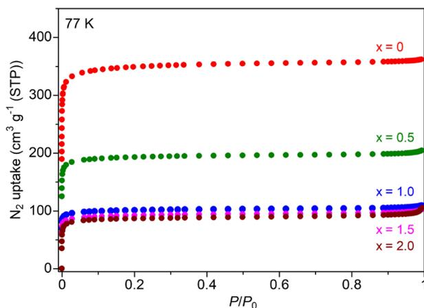
**Fig. 2** N<sub>2</sub> adsorption isotherms of UiO-66 ⊃ {Mg(TFSI)<sub>2</sub>}<sub>x</sub> (x = 0–2.0) at 77 K.
