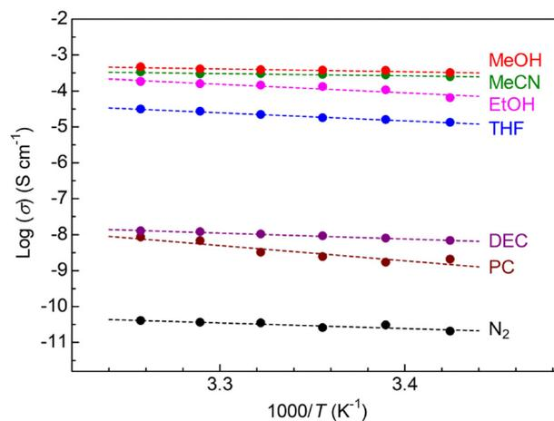
**Fig. 3** Temperature dependence of ionic conductivity of UiO-66 ⊃ {Mg(TFSI)<sub>2</sub>}<sub>1.0</sub> under various organic vapors.
