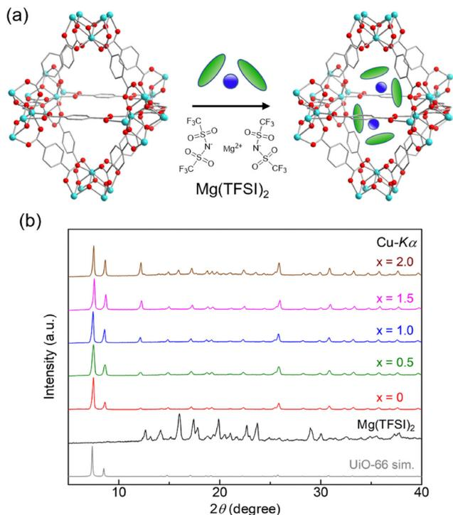
**Fig. 1** (a) Schematic illustration of the introduction of the Mg salts inside the pores of UiO-66. (b) XRPD patterns of bulk Mg(TFSI)<sub>2</sub> (precisely described as [Mg(H<sub>2</sub>O)<sub>6</sub>](TFSI)<sub>2</sub>·2H<sub>2</sub>O) and UiO-66 ⊃ {Mg(TFSI)<sub>2</sub>}<sub>x</sub> (x = 0–2.0).
