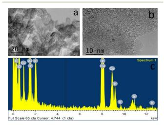
Fig. 9 A and B. HRTEM images of  $3@Al_2O_3$ -uncal after 45 h reaction at 350 °C with 0.10 mL min<sup>-1</sup> flow rate. A few particles, 2–3 nm in diameter are visible at higher magnification. The lattice spacing corresponds to metallic Ir. C. XEDS spectra of  $3@Al_2O_3$ -uncal after 45 h reaction.
