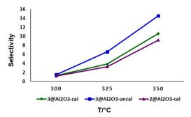
Fig. 6 Selectivity for P3 at different temperatures using various catalysts (selectivity =  $[P3/(P1 + P2 + P3)] \times 100$ ), flow rate = 0.09 mL min<sup>-1</sup>.
