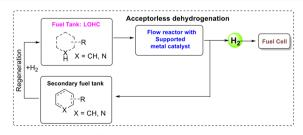
Fig. 1 Concept of LOHCs under continuous-flow conditions.
