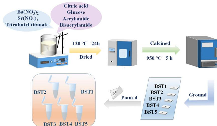
Fig. 1 The synthesis process of BST photocatalysts.
