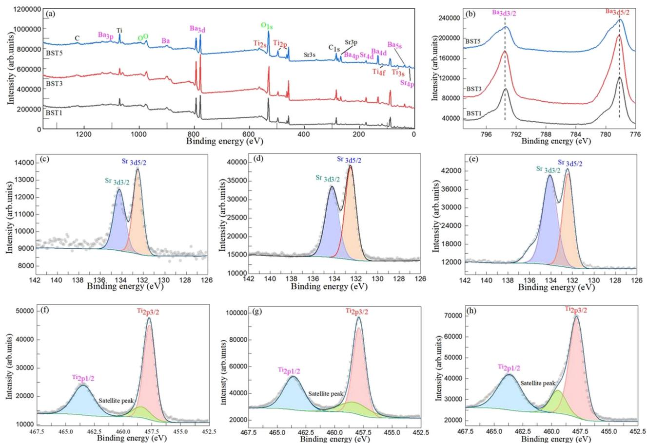
**Fig. 3** (a) XPS survey scan spectra and (b) Ba 3d spectra of the BST1, BST3 and BST5 photocatalysts. Sr 3d spectra of the (c) BST1, (d) BST3 and (e) BST5 photocatalysts. Ti 2p spectra of the (f) BST1, (g) BST3 and (h) BST5 photocatalysts.
