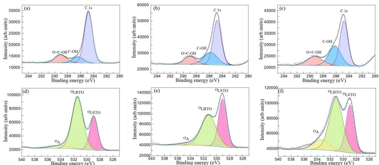
**Fig. 4** C 1s spectra of the (a) BST1, (b) BST3 and (c) BST5 photocatalysts. O 1s spectra of the (d) BST1, (e) BST3 and (f) BST5 photocatalysts.
