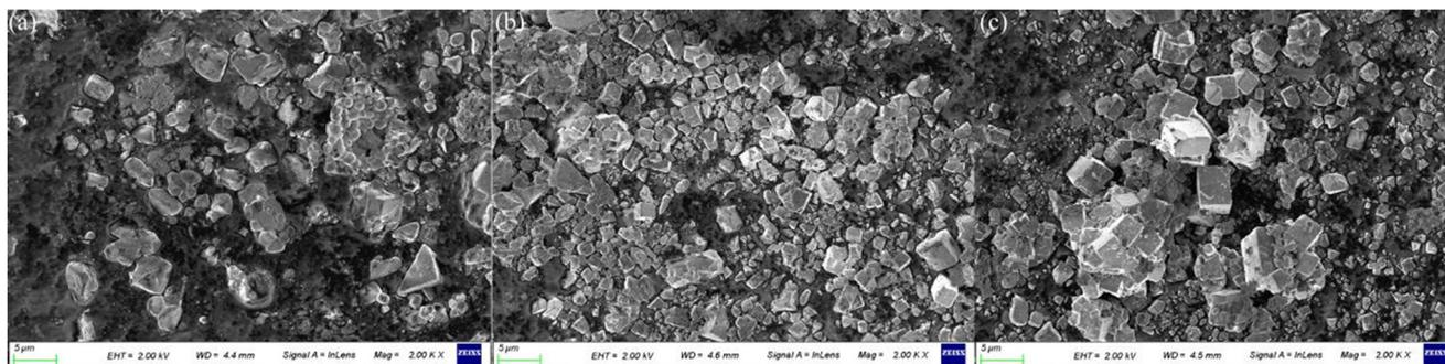
Fig. 5 SEM photographs of the (a) BST1, (b) BST3 and (c) BST5 photocatalysts.
