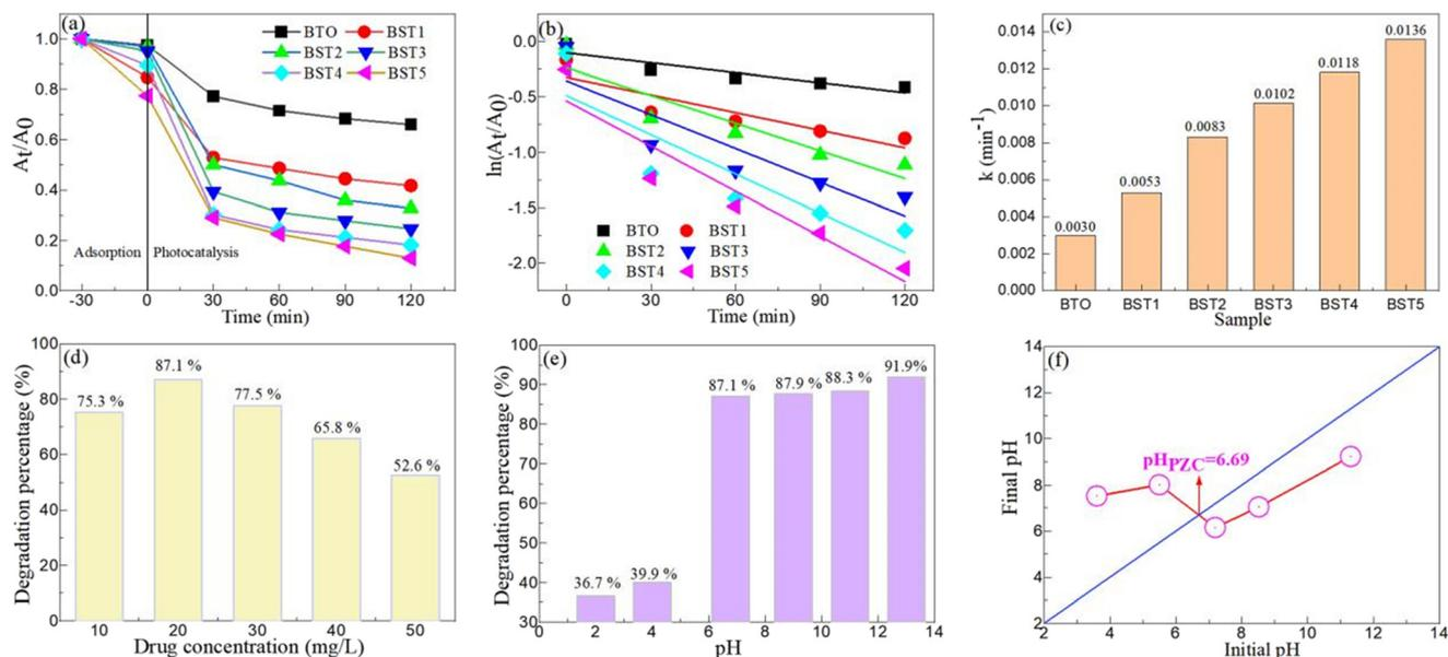
**Fig. 8** (a) The degradation efficiency for TC-HCl on the BST photocatalysts. (b) Plots of  $\ln(A_t/A_0)$  vs. irradiation time of the BST photocatalysts for the degradation of TC-HCl. (c) The apparent degradation rate constant ( $k$ ) value of the BST photocatalysts for the degradation of TC-HCl. Effects of (d) drug concentration and (e) pH value on the degradation of TC-HCl on the BST5 photocatalyst. (f) PZC of the BST5 photocatalyst.
