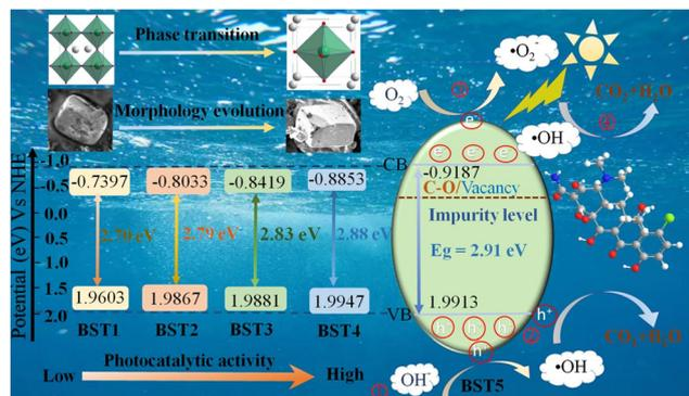
Fig. 10 The photocatalysis mechanism of the BST photocatalysts.
