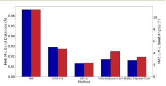
Fig. 5 Geometrical benchmarking results for the best-performing methods in each class (semi-empirical, extended tight binding, 3c and DFT), mean absolute error in metal-ligand bond length (blue) and ligand-metal-ligand bond angle (red), for the Cu\_benchmark\_set.
