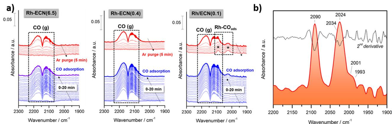
Fig. 3 a) Evolution of *in situ* DRIFT spectra during CO adsorption (20 min) and subsequent Ar purging (5 min) at 50 °C on Rh-ECN(6.5), Rh-ECN(0.4) and Rh/ECN(0.1) samples. b) DRIFT spectra recorded on Rh/ECN(0.1) sample after CO adsorption (20 min) and Ar purging (5 min) at 50 °C. The inclusion of second derivative curve facilitates the identification of the bands.
