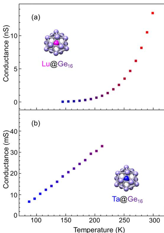
Fig. 10 Temperature dependent conductance of (a) Lu@Ge<sub>16</sub> and (b) Ta@Ge<sub>16</sub> assembled films.
