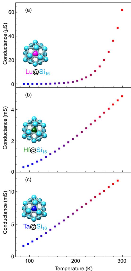
Fig. 8 Metal-atom dependence of temperature-dependent electrical conductance for different group-3, -4, and -5; (a) Lu@Si<sub>16</sub>, (b) Hf@Si<sub>16</sub>, and (c) Ta@Si<sub>16</sub> assembled films.
