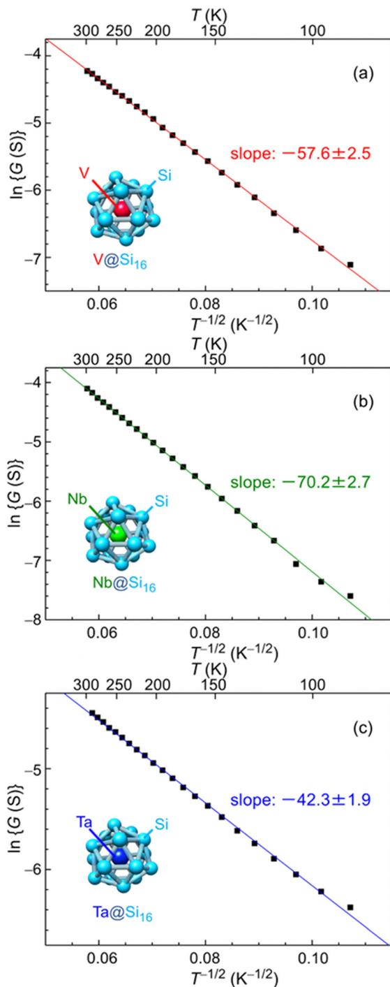
Fig. 7 Temperature dependent electrical conductance of  $M^V@Si_{16}$  ( $M^V =$  (a) V, (b) Nb, and (c) Ta) assembled films based on ES-VRH. Logarithm of conductance ( $\ln G$ ) versus  $T^{-1/2}$  for  $M^V@Si_{16}$  films is plotted at 87–300 K, and the slope values are shown in each. Reproduced with permission from ref. 33. Copyright 2021 American Chemical Society.
