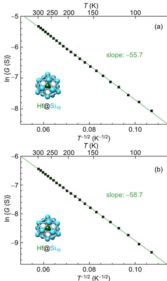
Fig. 9 Temperature dependent electrical conductance of a Hf@Si<sub>16</sub> assembled film based on the ES-VRH model; (a) as deposition and (b) after annealing at 423 K for 90 min in a vacuum. The logarithm of conductance ( $\ln G$ ) versus  $T^{-1/2}$  for Hf@Si<sub>16</sub> films is plotted at 87–300 K, and the slope values are shown in each.
