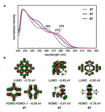
Fig. 5 Optoelectronic properties of **4T**, **5T**, and **6T**. (a) UV-vis absorption spectra of **4T**, **5T**, and **6T** in  $CH_2Cl_2$ . (b) Frontier molecular orbitals and the energy levels of **4T**, **5T**, and **6T** calculated at the B3LYP-D3/6-31G(d) level (isovalue = 0.03).
