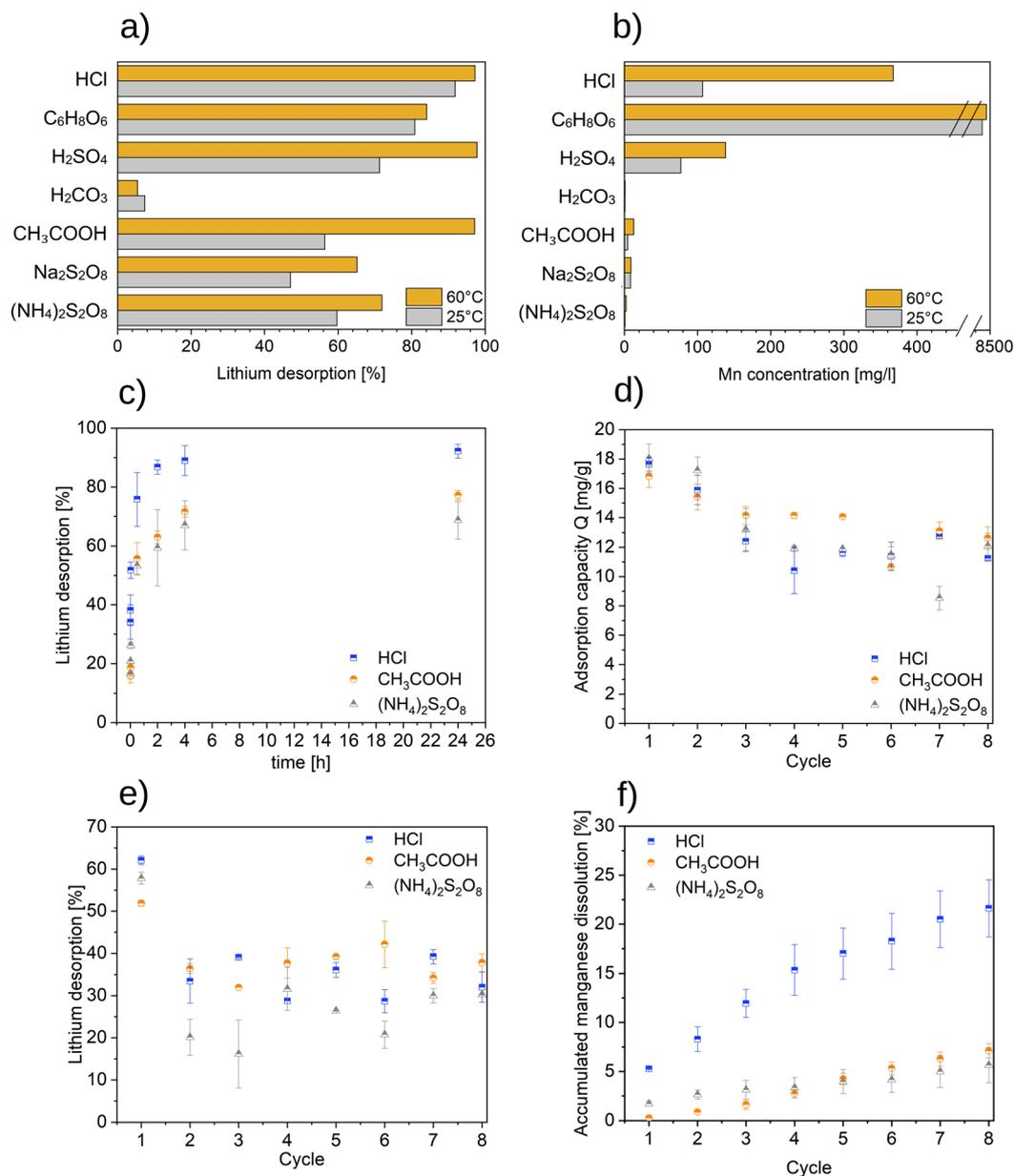
**Fig. 1** (a) ICP-OES Data of the Li recovery in preliminary desorption test using several desorption agents at 25 °C and 60 °C. (b) Mn dissolution in the preliminary tests using different desorption agents at 25 °C and 60 °C. (c) Li recovery over time using different desorption agents. (d) Cycle performance of adsorptions step using geothermal brine at 60 °C. (e) Cycle performance of Li recovery using various desorption agents at 60 °C. (f) Accumulated Mn dissolution over eight cycles.
