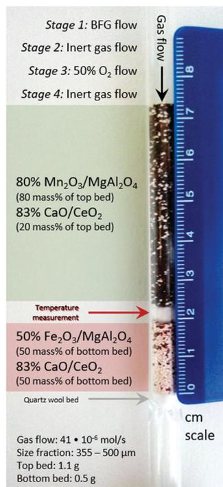
Fig. 3 Laboratory reactor bed to carry out the proof of concept experiments and experimental specifications. The scale bar on the right indicates the length in cm. Gas flow:  $41 \times 10^{-6} \text{ mol s}^{-1}$ . Size fraction of solids: 355–500  $\mu\text{m}$ . Top bed (manganese oxide and calcium oxide): 1.1 g. Bottom bed (iron oxide and calcium oxide): 0.5 g.
