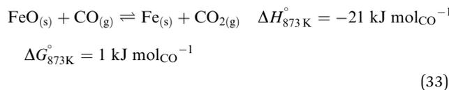
The higher carbon recovery comes at the cost of lower utilisation or oxidation of H<sub>2</sub> (eqn (34)) in the BFG (around 11% of inlet H<sub>2</sub> is oxidised when the reducer-carbonator is at 873 K). Higher H<sub>2</sub> utilisation is favoured at higher temperature (see Fig. S4 for an equilibrium diagram, ESI†) because of reduction of FeO and also due to increased favourability of the rWGS (eqn (1)).
