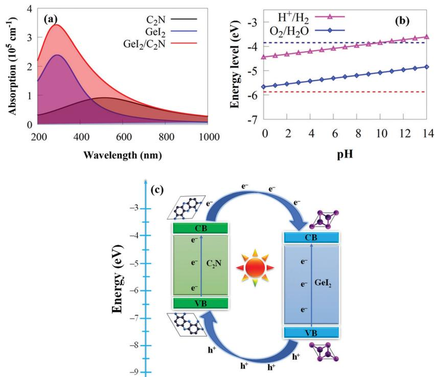
Fig. 6 (a) Calculated absorption spectra of the  $2 \times 2$  supercell of C<sub>2</sub>N, the  $4 \times 4$  supercell of GeI<sub>2</sub> and the GeI<sub>2</sub>/C<sub>2</sub>N vdW heterostructure. (b) The absolute energy bands for the conduction band minimum and valence band minimum of the GeI<sub>2</sub>/C<sub>2</sub>N vdW heterostructure with respect to pH (0–14). (c) Schematic diagram showing the transfer of photogenerated electrons and holes.
