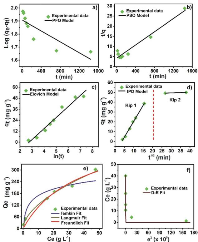
Fig. 6 (a) PFO; (b) PSO; (c) Elovich; (d) IPD kinetic model, (e) Langmuir, Freundlich, and Temkin isotherm fits; (f) Dubinin–Radushkevich isotherm for Hg(II) adsorption onto Zr-MOF@Fe<sub>3</sub>O<sub>4</sub>.
