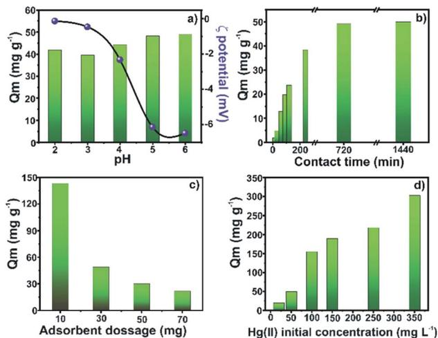
Fig. 4 Effect of (a) pH; (b) contact time; (c) adsorbent dosage; (d) Hg(II) concentration on the adsorption capacity of Zr-MOF@Fe<sub>3</sub>O<sub>4</sub>. Conditions: mass of Zr-MOF@Fe<sub>3</sub>O<sub>4</sub> = 30 mg, [Hg(II)] = 50 mg L<sup>-1</sup>, volume = 30 mL, time = 12 h (change accordingly).
