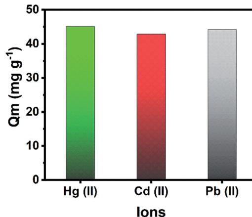
Fig. 5 Simultaneous removal of Hg(II), Cd(II), and Pb(II) from a ternary metal solution. Conditions: mass of Zr-MOF@Fe<sub>3</sub>O<sub>4</sub> = 30 mg, [ion] = 50 mg L<sup>-1</sup> each, volume = 30 mL, time = 12 h.
