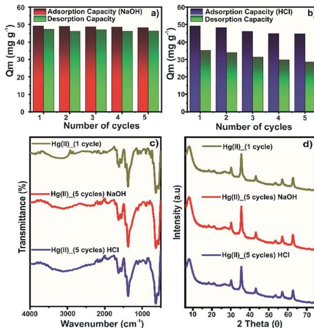
Fig. 8 Regeneration and reusability tests of Zr-MOF@Fe<sub>3</sub>O<sub>4</sub> for the removal of Hg(II) with (a) NaOH eluent and (b) HCl eluent; (c) FTIR spectra; (d) PXRD patterns of Zr-MOF@Fe<sub>3</sub>O<sub>4</sub> after reusability tests. Conditions: mass of Zr-MOF@Fe<sub>3</sub>O<sub>4</sub> = 30 mg, [Hg(II)] = 50 mg L<sup>-1</sup>, [NaOH]/[HCl] = 0.1 mol L<sup>-1</sup>, volume = 30 mL, time = 12 h.
