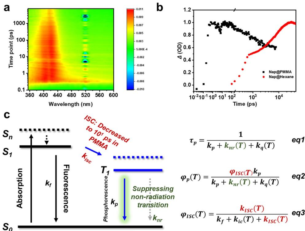
Fig. 3 (a) Transient absorption two-dimensional temporal evolution spectra at room temperature of Nap@PMMA; (b) transient absorption traces of Nap@PMMA at 421 nm and naphthalene in hexane at 412 nm; (c) schematic illustration of a Jablonski diagram for long-lived RTP of the phosphor in our system.
