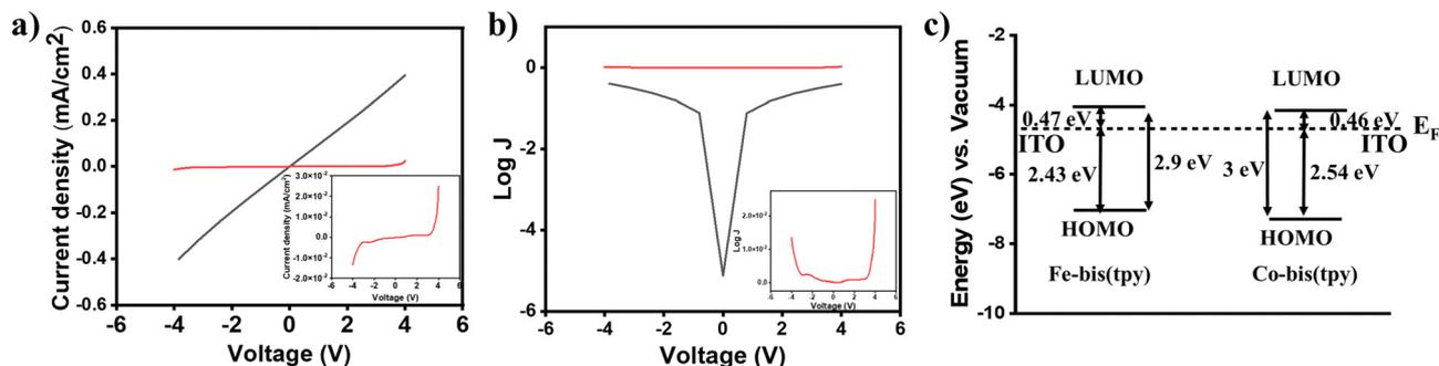
Fig. 6 (a) A comparison of the  $J$ - $V$  plot of a reference junction (solid black line) and that of a molecular junction (solid red line). (b)  $\text{Log } J$  vs. voltage plots and (c) energy level diagrams of ITO ( $E_F$  4.7 eV) and the HOMO and LUMO energies of  $\text{Fe}^{2+}$ -bis(tpy) and  $\text{Co}^{2+}$ -bis(tpy).
