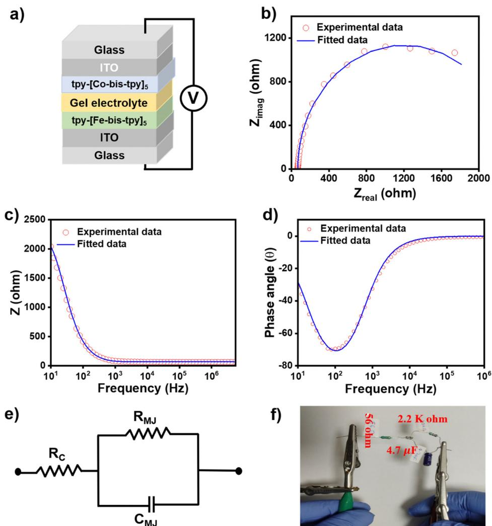
Fig. 7 (a) A schematic description of a molecular junction composed of ITO/tpy-[Fe(bis-tpy)]<sub>5</sub>/gel electrolyte/[Co(bis-tpy)]<sub>5</sub>-tpy/ITO. (b) The Nyquist plot of the junction. (c and d) Bodes plot at varying frequencies. (e) The Randles equivalent circuit and (f) a real circuit for the experimental validation of the fitted model.
