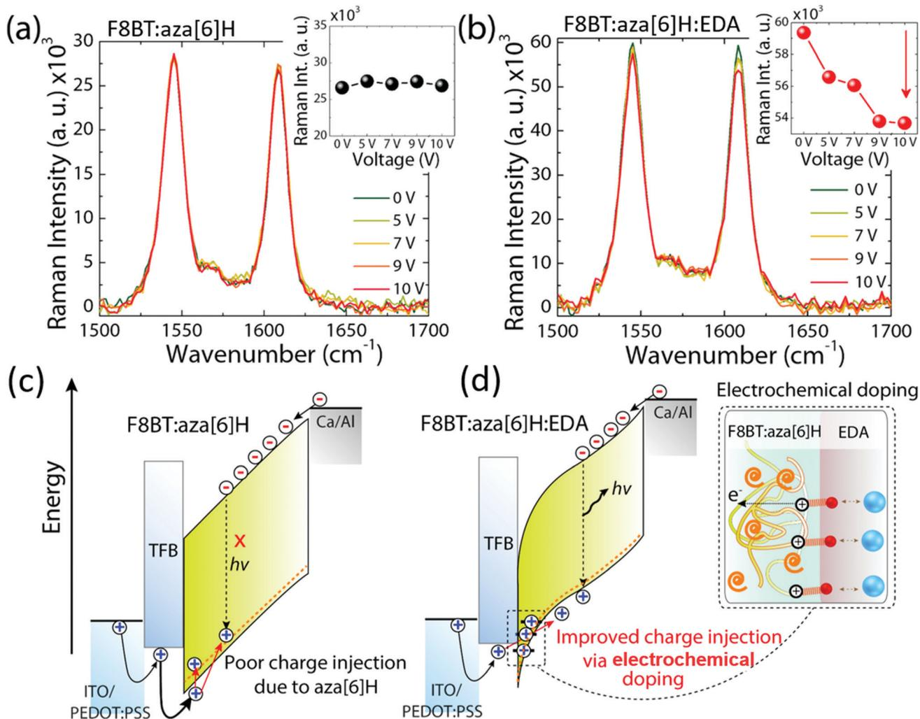
Fig. 5 (a) and (b) *In situ* electric-field-dependent Raman spectra of the F8BT:aza[6]H and F8BT:aza[6]H:EDA devices, respectively. The inset figures indicate the changes in the selective Raman peaks at 1608 cm<sup>-1</sup> under an electric field ranging from 0 V to 10 V. (c) and (d) The proposed mechanism of poor charge injection in F8BT:aza[6]H and improved charge injection and charge balance in an EDA-doped device via the electrochemical doping by EDA molecules (inset), respectively.
