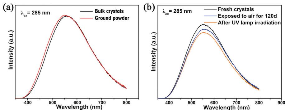
Fig. 4 (a) PL spectra of bulk crystals and ground powder for  $\text{Cs}_2\text{Cd}_2\text{BrCl}_5$ , and (b) emission spectra of fresh  $\text{Cs}_2\text{Cd}_2\text{BrCl}_5$  crystals, crystals exposed to air for 120 d, and after 12 h of UV-lamp irradiation.
