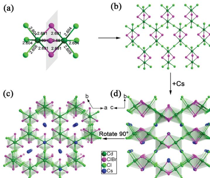
**Fig. 1** (a) Coordination of  $\text{Cd}_2\text{Cl}_6(\text{Br/Cl})_3$  dimers and their bond lengths; (b) 2D layer structure built from adjacent  $\text{Cd}_2\text{Cl}_6(\text{Br/Cl})_3$  dimers that are inter-linked by sharing the Cl atoms along the  $ac$  plane; (c) crystal structure of  $\text{Cs}_2\text{Cd}_2\text{BrCl}_5$  viewed along the  $ab$  plane; and (d) crystal structure of  $\text{Cs}_2\text{Cd}_2\text{BrCl}_5$  viewed along the  $bc$  plane.
