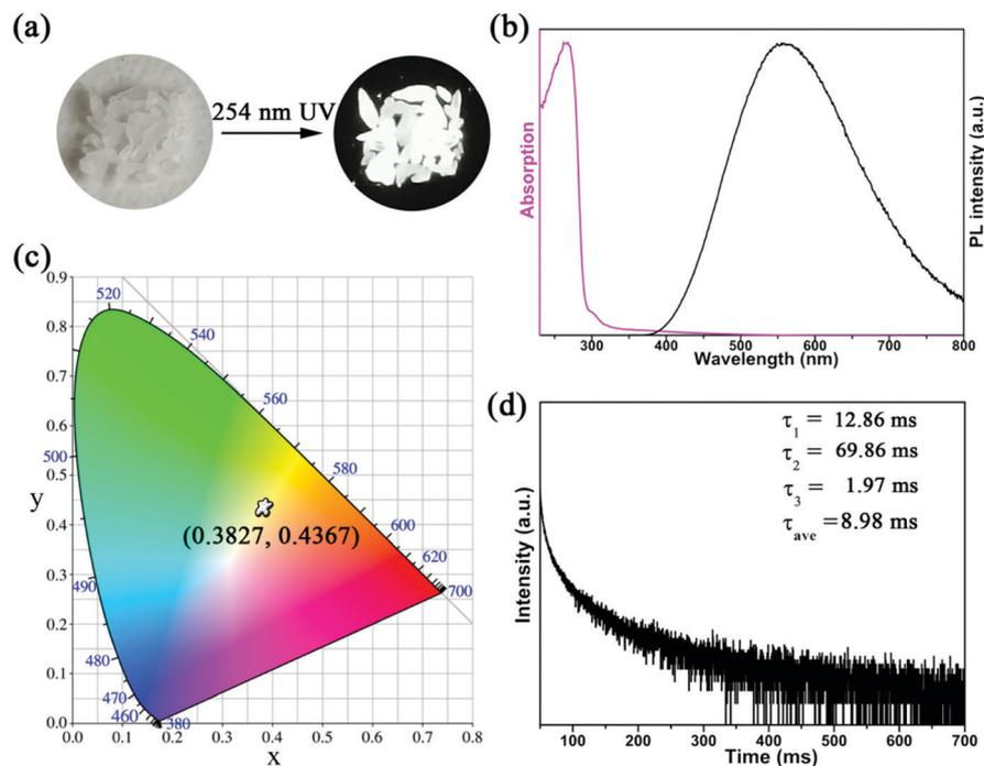
Fig. 3 PL properties of compound  $\text{Cs}_2\text{Cd}_2\text{BrCl}_5$  at room temperature: (a) images of  $\text{Cs}_2\text{Cd}_2\text{BrCl}_5$  crystals under ambient light and 254 nm UV-light excitation, (b) UV-vis absorption spectrum (purple line) and emission spectrum (black line), (c) CIE chromaticity coordinates, and (d) lifetime decay curve.
