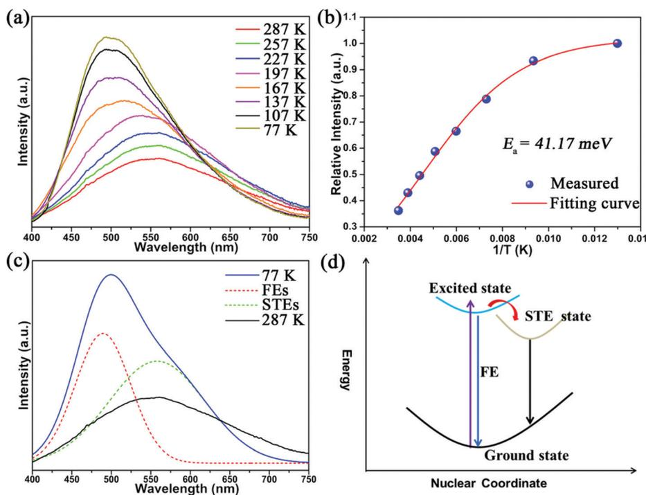
Fig. 5 (a) Temperature-dependent emission spectra; (b) functional relationship between  $1/T$  and the integrated PL intensity; (c) emission spectrum at 77 K (solid blue line) and 287 K (solid black line), with the emission spectra of FEs (red dashed line) and STEs (green dashed line) obtained *via* Gaussian fitting to split the emission spectrum at 77 K; and (d) corresponding emission mechanism configuration diagram of  $\text{Cs}_2\text{Cd}_2\text{BrCl}_5$ .
