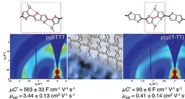
Fig. 8 Sections of chemical structures of **pgBTTT** and **p(g2T-TT)** addressing S–O interactions with corresponding GIWAXS maps. Reproduced from ref. 78 with permission from the American Chemical Society.
