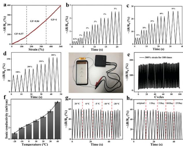
**Fig. 8** The sensing performance of ionogel: (a) the variation of  $\Delta R/R_0$  against the strain (gauge factor); the variation of  $\Delta R/R_0$  at (b) 0.5% to 5%; (c) 5% to 50%; (d) 150% to 300%; (e) 300% for 100 cycles; (f) the conductivities of ionogel at different temperatures; the comparison of the sensing signal at (g) different temperatures; (h) different storage time periods at  $-20^\circ\text{C}$ .
