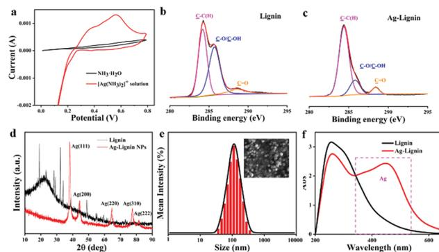
Fig. 2 Characterizations of the Ag-Lignin NPs: (a) CV curves of the [Ag(NH<sub>3</sub>)<sub>2</sub>]<sup>+</sup> solution; (b and c) XPS spectra in the C 1s regions of Lignin and Ag-Lignin; (d) XRD patterns of the Lignin and Ag-Lignin; (e) DLS analysis of the Ag-Lignin and SEM photo of Ag-Lignin NPs; (f) UV-vis spectra of Lignin and Ag-Lignin.
