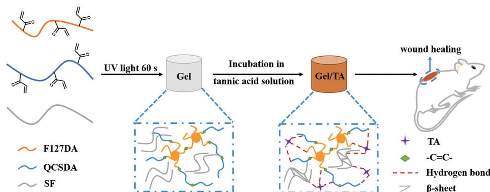
Scheme 1 A schematic diagram of Gel/TA hydrogel adhesive fabrication.
