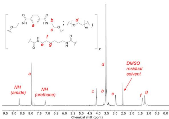
Fig. 2 <sup>1</sup>H NMR of the 1BHETA:2PEG polyurethane in d<sub>6</sub>-DMSO.
