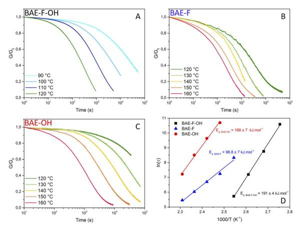
Fig. 4 Normalized stress-relaxation curves at different temperatures for a 1% strain (A) for BAE-F-OH, (B) for BAE-F and (C) for BAE-O. (D) Fitting of the relaxation time ( $\tau$ ) vs. temperature data by the Arrhenius equation for BAE-F-OH (black squares), BAE-F (blue triangle) and BAE-OH (red circles).
