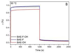
(A) Normalized stress relaxation of BAEs at 120 °C for a 1% strain (B) creep and recovery data for BAEs at 50 °C for an applied stress of 2 kPa.
