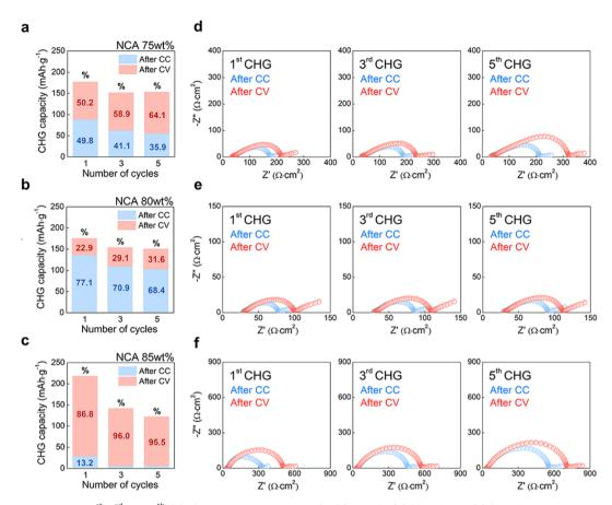
Fig. 5 Representation of the 1st, 3rd, and 5th CC-CV charge capacity of NCA (a) 75 wt%, (b) 80 wt% and (c) 85 wt% composite cathodes with CC charging (bluish bar chart) to 3.7 V vs. In/InLi at 0.5C followed by CV charging (reddish bar chart) with a cut-off condition of 0.05C. Nyquist plots of after the 1st, 3rd, and 5th CC (bluish open dots) and CV (reddish open dots) with respect to content of NCA (d) 75 wt%, (e) 80 wt%, and (f) 85 wt%.
