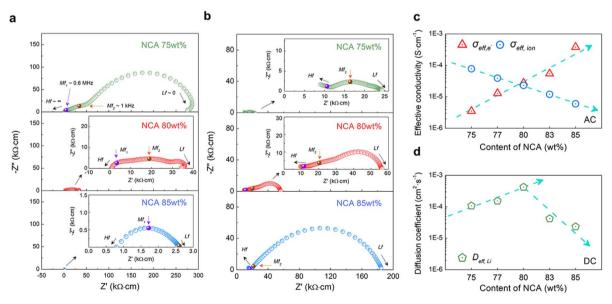
Fig. 4 Nyquist plots of (a) ion-blocking cells [SS||composite cathode||SS|| and (b) electron-blocking cells [Li||LPSC l||composite cathode||LPSC l||Li] with 75 wt%, 80 wt%, and 85 wt% of NCA in composite cathodes. (c) Effective conductivity ( $\sigma_{eff}$ ) and (d) diffusion coefficients ( $D_{eff,Li}$ ) results of the composite cathode extracted from EIS and DC polarization measurements as a function of NCA content from 75 wt% to 85 wt%.
