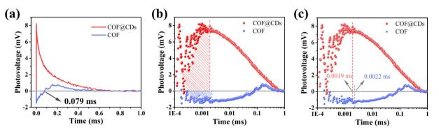
Fig. 7 (a) The transient photovoltage curves, the corresponding (b) amount of charge extraction and (c) maximum charge extraction time of the COF and COF@CDs.
