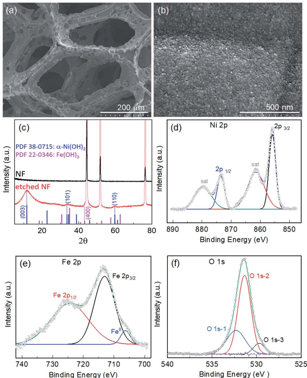
Fig. 1 SEM images of nickel foam (NF) etched for 18 h (Fe-18h/NF) in an ethanolic  $\text{FeCl}_3$  solution at  $50^\circ\text{C}$ : (a) surface view showing microporous Ni backbones at low magnification, and (b) a high-magnification view showing hierarchically-structured metallic Fe@Ni-Fe-hydroxide nanoparticles with a diameter of  $\sim 10$  nm. (c) XRD patterns of pristine NF and NF etched for 18 h. XPS spectra of (d) Ni 2p, (e) Fe 2p, and (f) O 1s for the Fe-18h/NF sample.
