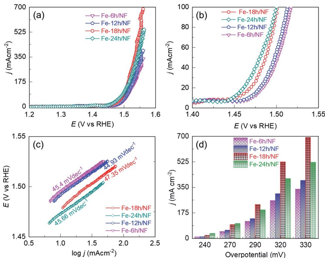
Fig. 3 Comparison of the electrocatalytic performance of the etched NF in a 1 M KOH solution:  $iR$  compensated anodic linear sweep voltammograms (LSVs) of the (a) NFs etched for 6, 12, 18, and or 24 h, (b) magnified view of (a) below 100 mA cm<sup>-2</sup>, (c) corresponding Tafel slopes extracted from the LSVs, and (d) current density profiles with respect to the OER overpotential.
