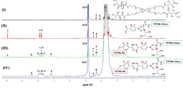
Fig. 4 <sup>1</sup>H NMR spectra in D<sub>2</sub>O buffered at pD = 8.5 of (I) the starting TP10k-Gluco, (II) the fully-formed (within 1 h) adduct of TP10k-Gluco with a stoichiometric amount of FPBA, and (III and IV) the "boronate" hydrogel formed from the reaction of the TP10k-Gluco-FPBA adduct with a stoichiometric amount of TP10k-Hz after three days (III) and after seven (IV).
