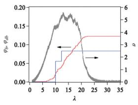
Fig. 12 Evolution of the broken strand fraction  $\varphi_b$  (red curve) during stretch for a 1a3-6505 network. Blue line indicates the broken double linkage fraction  $\varphi_{db}$ . The gray curve shows the stress for comparison.
