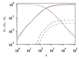
Fig. 3 Time development of number fraction of the arms. Dotted, solid, and broken curves are unreacted dangling ones  $\varphi_{a}$ , the fraction involved in single linkages  $\varphi_{s}$ , and those contributed as double linkages  $\varphi_{d}$ , respectively. Black and red curves are for 2a2-3802 and s2020, respectively.
