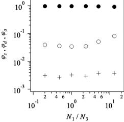
Fig. 4 Arm fractions in dangling ends  $\varphi_a$  (cross), single linkages  $\varphi_s$  (filled circle), and double linkages  $\varphi_d$  (unfilled circle) in the resultant networks for 2a2 and 1a3 systems.
