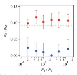
Fig. 13 Broken strand fraction in the final fractured networks  $\varphi_b$  (red) and the fraction of broken double linkages to all the embedded double linkages  $\varphi_{db}$  (blue) against the arm length ratio for 2a2 (top) and 1a3 (bottom) systems. Horizontal broken lines indicate the value for Rnd. Error bars correspond to the standard deviation for 8 independent simulation runs.
