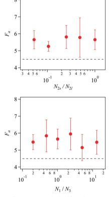
Fig. 11 Apparent fracture energy obtained from the stress-stretch curves plotted against the arm length ratio for 2a2 (top) and 1a3 (bottom) systems. Horizontal broken lines indicate the value for Rnd. Error bars correspond to the standard deviation for 8 independent simulation runs.
