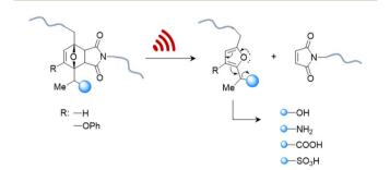
Fig. 4 US-induced cargo release from 2-furylcarbinol mechanophore *via* retro Diels–Alder reaction followed by fragmentation cascade.<sup>87</sup> The cargo scope includes alcohols (aryl/alkyl), amines (aryl/alkyl), carboxylic acids, and sulfonic acids.
