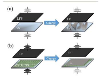
Fig. 10 Schematic illustrations of the Li electrodeposition process on the (a) stainless steel (SS) and (b) mesoporous silica thin films with channels perpendicular to the stainless steel substrate (MSTF⊥SS) in the anode-free Li metal batteries. Reproduced with permission from ref. 79.
