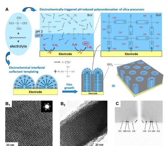
Fig. 3 (A) Schematic illustration of the EASA process. (B) TEM images of the ordered and oriented mesoporous silica film ( $B_1$  top view with electron diffraction pattern as inset;  $B_2$  cross-section). (C) Typical GI-XD pattern confirming the hexagonal packing of vertically aligned mesopore channels. Reproduced with permission from ref. 40.
