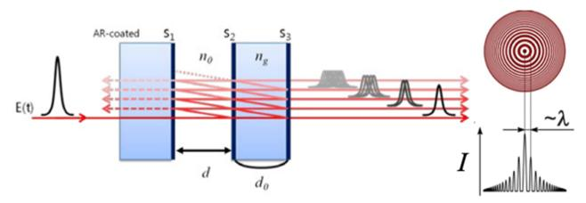
Illustration of the working principle of a Fabry-Perot interferometer and a typical Fabry-Perot interference pattern.
