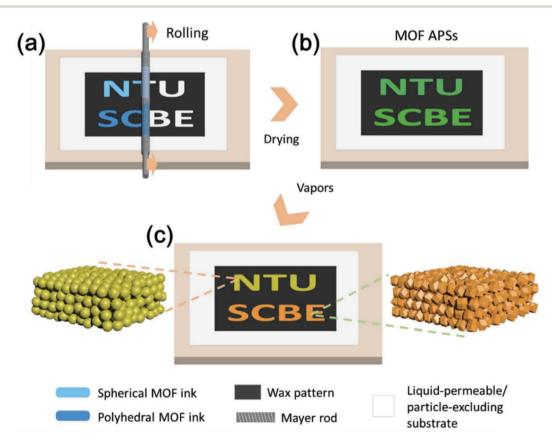
Fig. 11 Illustration of Mayer rod coating of a MOF amorphous photonic structure (APS). (a) Selective wetting of the hydrophilic area of the substrate during coating with spherical/polyhedral MOF inks; (b) formation of APS patterns of spherical or polyhedral MOF particles after the removal of water; (c) vapour-responsive colour changes of the MOF APS patterns.<sup>175</sup>
