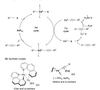
**Scheme 4** (a) General proposed mechanism for Sonogashira cross-coupling reactions. (b) Synthetic models reported in the literature.
