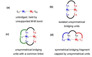
Scheme 2 Commonly used motifs for unsymmetrical ligand scaffold design in heterobi- or multimetallic complexes: (a) unbridged complexes supported by mononucleating ligands and held by metalmetal interactions; (b) complexes containing one or more isolated unsymmetrical bridging units; (c) complexes in which several bridging units are linked with a common linker; (d) heterobimetallic complexes containing a bridging fragment capped by unsymmetrical coordinating units
