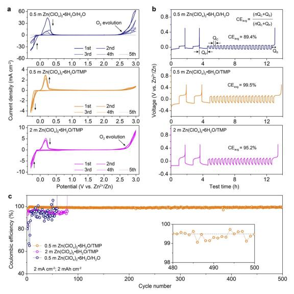
Fig. 4 Electrochemical reversibility of the Zn electrode. (a) CV profiles of Zn//Ti cells in different electrolytes from -0.3 to 3.0 V at 1 mV s<sup>-1</sup>. (b) Voltage profiles of Zn//Cu cells in different electrolytes using a 'reservoir half-cell' method. (c) Zn plating/stripping CE of Zn//Cu cells with electrolytes of 0.5 m H<sub>2</sub>O, 0.5 m TMP, and 2 m TMP at 2 mA cm<sup>-2</sup> and 2 mA h cm<sup>-2</sup>. The inset magnifies the profile within 480–500 cycles.
