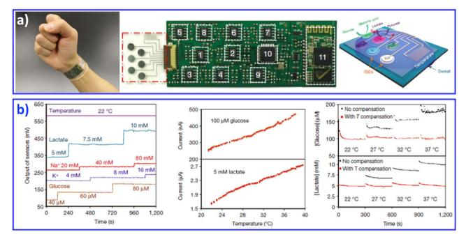
Fig. 8 A FISA integrating a multiplexed sweat sensor array and a wireless flexible printed circuit board FPCB for the simultaneous and selective screening of a panel of biomarkers in sweat. (a) Images and schematic illustrations of the FISA. (b) System-level characterization of the sensor array. Reproduced with permission from ref. 28. Copyright 2016, Nature Publishing Group.
