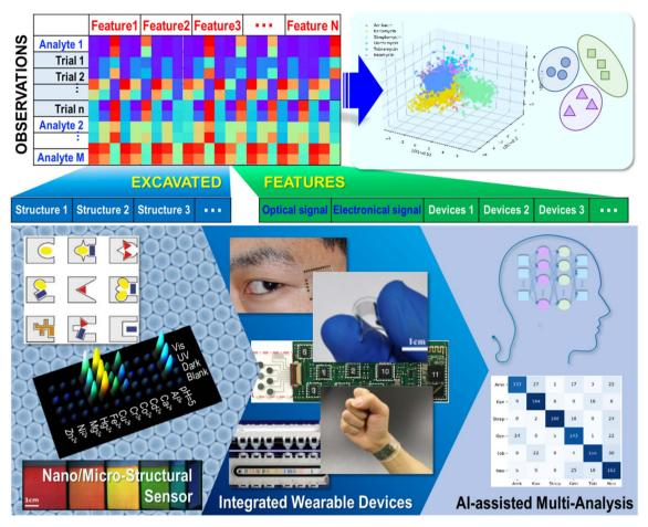
Fig. 1 Schematic of promoted multi-analyte discriminative sensing *via* structural diversity, wearable device integration, and artificial intelligence (AI) assisted strategies. Reproduced with permission from ref. 17, 28, 40, 68, 73, 117, 128 and 129. Copyright 2001, Wiley-VCH. Copyright 2016, Nature Publishing Group. Copyright 2015, Nature Publishing Group. Copyright 2016, Wiley-VCH. Copyright 2015, ACS publishing group. Copyright 2021, Wiley-VCH. Copyright 2022, ACS publishing group.
