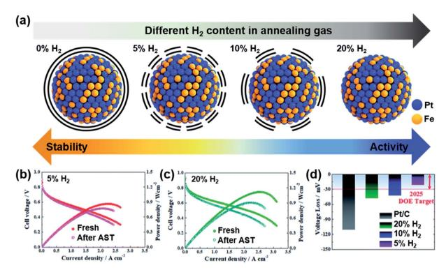
Fig. 5 (a) Difference in the carbon shell depending on annealing conditions; various percentages of  $H_2$  flow were used at 700 °C. I-V curves before and after accelerated stress tests (ASTs) performed under (b) 5%  $H_2$  and (c) 20%  $H_2$ . (d) Voltage loss at 0.8 A cm<sup>-2</sup> after ASTs. Reproduced from ref. 90 with permission, copyright 2021, the Royal Society of Chemistry.
