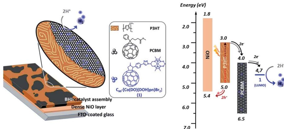
Fig. 1 Representation (left) and energy diagram (right) of a photocathode for  $\text{H}_2$  evolution based on a PCBM:P3HT bulk heterojunction BHI combined with the cobalt diimine-dioxime – fullerene assembly **1** as  $\text{H}_2$ -evolving catalyst (see ESI† and ref. 30 for energy values).
