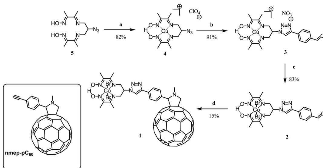
Scheme 1 Synthesis of the cobalt diimine-dioxime – fullerene assembly **1**; (a)  $\text{Cu}(\text{ClO}_4)_2 \cdot 6\text{H}_2\text{O}$ , acetone, RT; (b) 4-ethynylbenzaldehyde,  $N, N', N'', N'''$ -pentamethyldiethylenetriamine,  $\text{CuBr}$ ,  $\text{MeOH}$ , Ar,  $50 \text{ }^\circ\text{C}$ , 3.5 h; (c)  $\text{CoBr}_2$ ,  $\text{O}_2$ , RT, 2 h; (d)  $\text{C}_{60}$ , sarcosine, toluene:1,2-dichloroethane 2:1, Ar, reflux, 5 h; inset: structure of  $\text{nmep-pC}_{60}$ .
