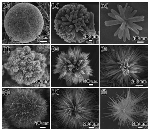
Fig. 7 SEM images of 3D nanotree composed of (a–c) nanorods (d–f) nanoribbons (g–i) nanowires.<sup>100</sup>
