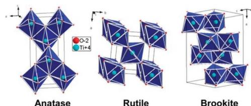
Fig. 1 Anatase, rutile, and brookite crystal structure of TiO<sub>2</sub>.<sup>10</sup>
