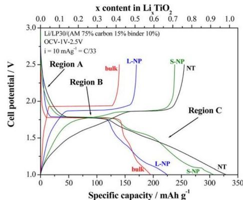
Fig. 2 The voltage–capacity curves of anatase  $\text{TiO}_2$ .<sup>11</sup>
