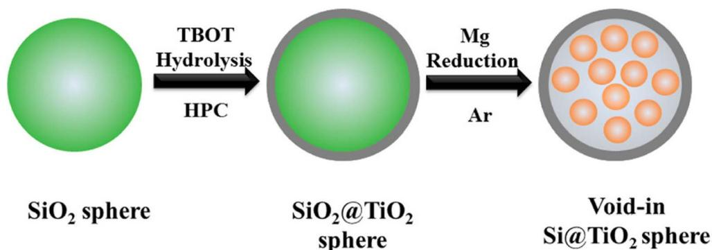
Fig. 9 Schematic diagram of the preparation process of Si@TiO<sub>2</sub> composite.<sup>121</sup>
