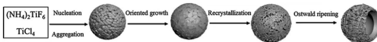
Fig. 6 Schematic illustration of the probable formation mechanism of hollow porous TiO<sub>2</sub> microspheres.<sup>97</sup>
