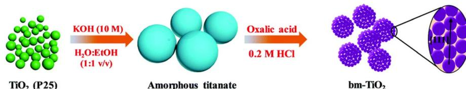
Fig. 3 Preparation process of mesomorphic  $\text{TiO}_2$  with brookite phase.<sup>39</sup>
