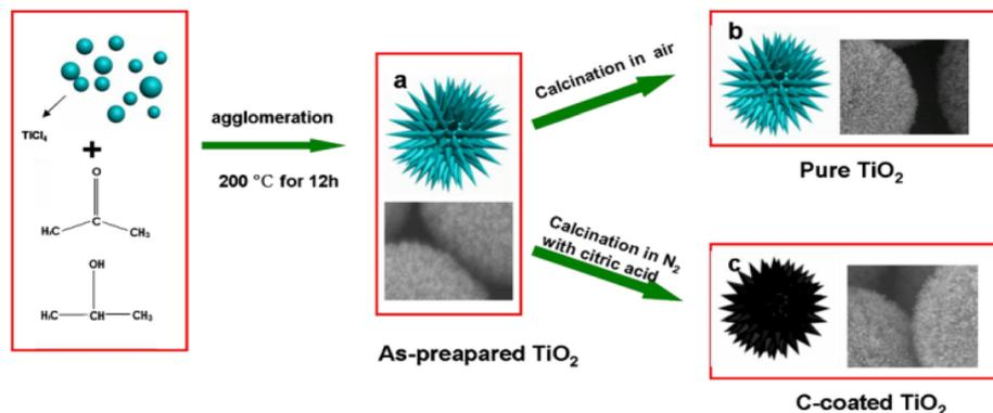
Fig. 5 Schematic diagram of the growth mechanism of TiO<sub>2</sub> microspheres.<sup>94</sup>
