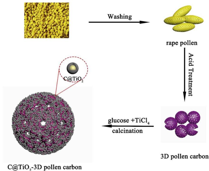
Fig. 8 Schematical illustration of the synthetic process of C@TiO<sub>2</sub>/3D pollen carbon.<sup>114</sup>
