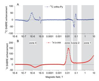
Fig. 9 (A)  $^{13}$ C SABRE field dependence for ortho carbon of  $^{15}$ N-pyridine, for details see ref. 142. (B)  $^{1}$ H SABRE field dependence for hydride protons on ImesIr-catalyst (unpublished results provided by A. Kiryutin).
