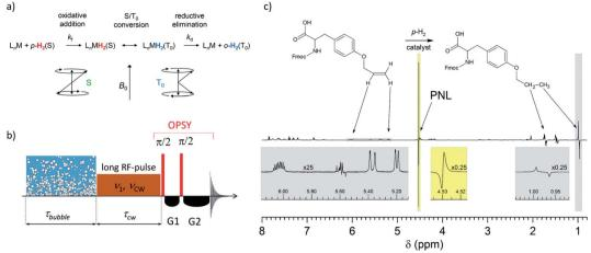
Fig. 10 (a) Magnetic conversion of p-H<sub>2</sub> (spin state S) to o-H<sub>2</sub> in spin state  $T_0$ . (b) The PANEL (PArtially NEgative Line) experiment for the indirect detection of the hydrogen catalyst complex. (c) <sup>1</sup>H NMR PHIP spectrum recorded during the hydrogenation with p-H<sub>2</sub> of Fmoc-O-allyl-tyrosine (left) to Fmoc-O-propyl-tyrosine (right), showing a strong PNL signal at 4.53 ppm (for details see Kiryutin *et al.*<sup>93</sup>).
