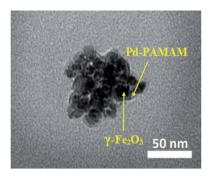
Fig. 3 TEM images of the PAMAM  $G_0$ -Pd@ $\gamma$ -Fe $_2O_3$  complex.
