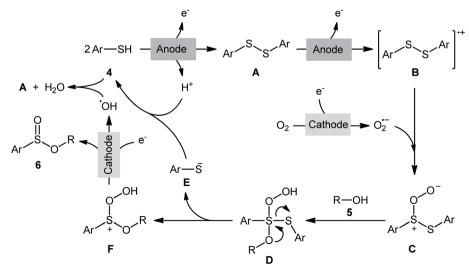
Scheme 3 Proposed mechanism for electrosynthesis of sulfinic esters 6.
