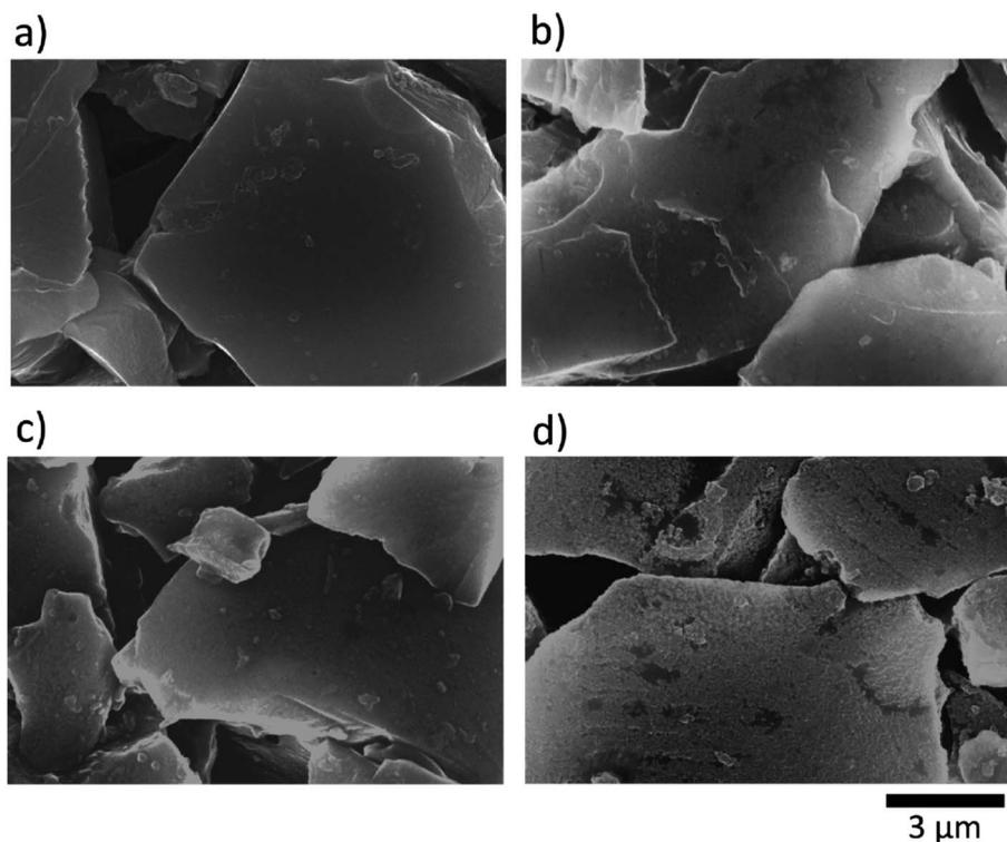
Fig. 4 SEM images for hard-carbon electrodes; (a) pristine, and (b–d) after the first reduction–oxidation cycle test in PC-based electrolyte solutions (b) without and (c and d) with (c) 2 vol% and (d) 10 vol% FEC at a rate of 25 mA g<sup>-1</sup> in the coin-type Na cells.<sup>70</sup> Copyright 2014, Elsevier B. V.
