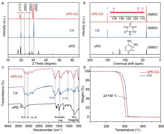
Fig. 1 (a) Powder XRD patterns, (b) <sup>13</sup>C-NMR spectra, (c) FTIR spectra of as-synthesized oPD-CA, pristine CA, and oPD, and (d) TG curves of oPD-CA, and the pristine CA in the nitrogen environment.
