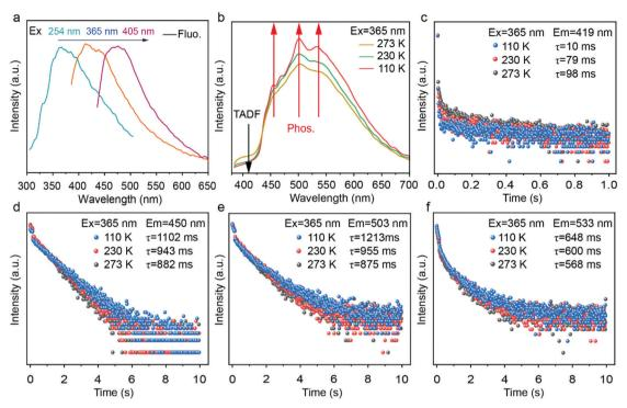
Fig. 3 (a) Excitation wavelength dependent room-temperature fluorescence spectra, (b) temperature-dependent afterglow spectra, (c) TADF decay kinetics, (d) phosphorescence decay kinetics for 503 nm, and (f) phosphorescence decay kinetics for 533 nm.
