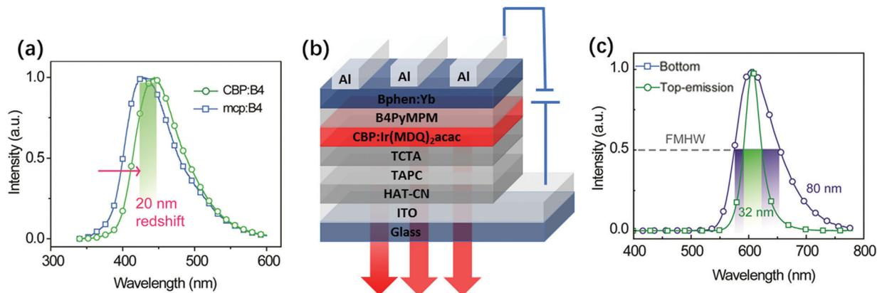
**Fig. 1** (a) PL spectra of CBP: B4PyMPM and mCP:B4PyMPM in films at 300 K. (b) Device structure of the bottom-emitting device. (c) Normalized EL spectra of the top-emitting and bottom-emitting devices.
